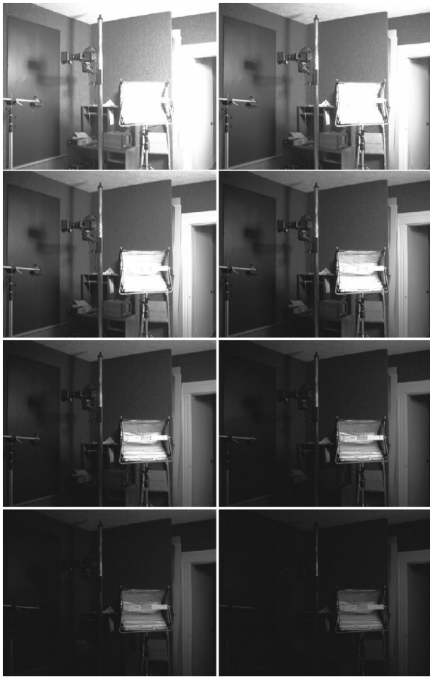
Fig. 1 “Studio” scene. Eight pictures of a static scene taken at different exposure times, photographed using a Nikon E2N digital camera with aperture f/6.7 . The original image resolution is 1280 \times 1000 . The exposure times are, from brightest to darkest, \frac{1}{8} , \frac{1}{15} , \frac{1}{30} , \frac{1}{60} , \frac{1}{125} , \frac{1}{250} , \frac{1}{500} , and \frac{1}{1000} s.
