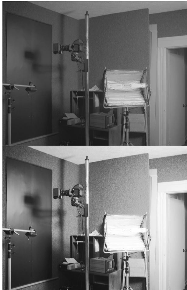
Fig. 9 High dynamic range output images for the Studio scene. Top: Results after gamma modification, \gamma=0.01 , and \epsilon=0.001 . Bottom: Results after histogram equalization.
